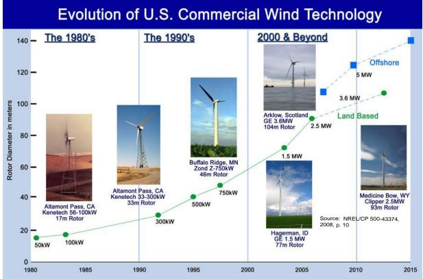
Figure 2-4. Increasing Size of Utility-scale Turbines from 1980 to the Present and Beyond
