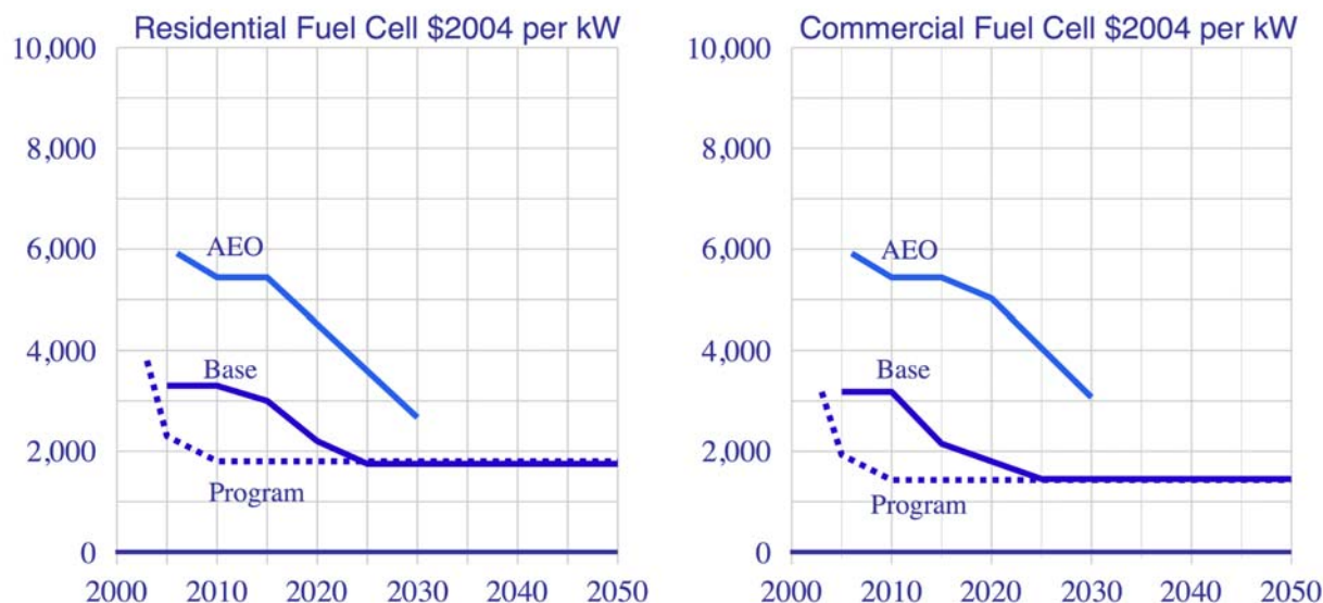
Figure 3.12. Projected Capital Cost of Stationary Fuel Cell Systems for the AEO2006 Reference, GPRA Base, and GPRA HFCIT Program Cases
