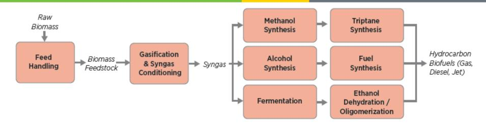
Biomass feedstocks are gasified to produce a clean syngas, which is used as a feedstock for hydrocarbon biofuel production.
