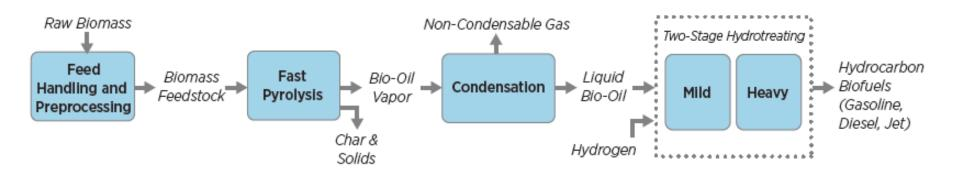
Biomass is rapidly heated in a fluidized bed reactor to yield vapors, which are condensed into a liquid bio-oil. This bio-oil is subsequently hydroprocessed to produce hydrocarbon biofuel blendstocks.
