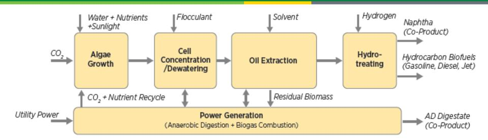
Bio-oil is extracted from algal biomass via high-pressure homogenization and a hexane solvent; the algal oil can then be hydrotreated to produce advanced hydrocarbon fuels.
