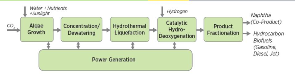
Bio-oils are separated from water via heat and pressure, so they can be catalytically hydrotreated and converted to advanced hydrocarbon fuels.
