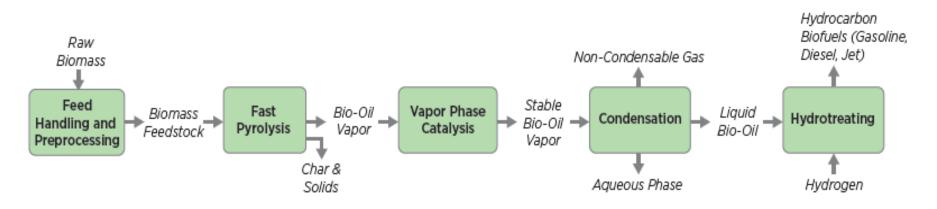
Biomass is rapidly heated in a fluidized bed reactor containing a catalyst to yield vapors, which are catalytically modified and condensed into a partially stabilized and deoxygenated liquid bio-oil. This stable bio-oil is subsequently upgraded to produce hydrocarbon biofuel blendstocks.
