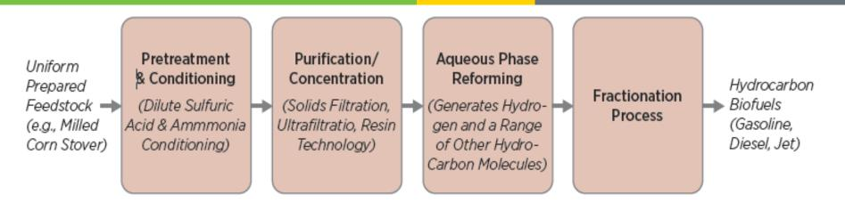
Biomass-derived sugars—separated from feedstock through a series of chemical and biochemical processes—are upgraded via aqueous phase reforming into hydrocarbons for fuels and co-product commodities.
