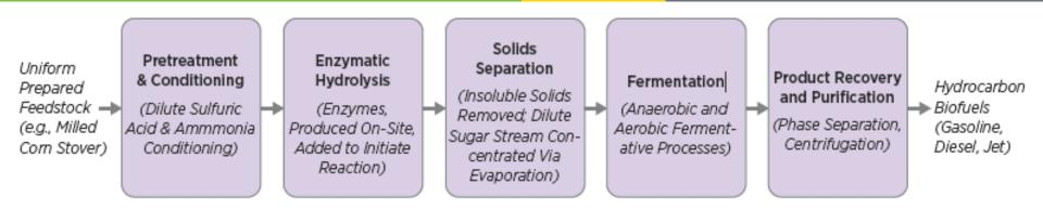
Biomass-derived sugars—separated from feedstocks through a series of chemical and biochemical processes—are further transformed, recovered, and purified to yield hydrocarbons for fuels and co-product commodities.
