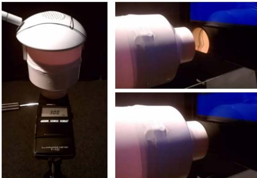
Figure 1.5.1 Light source directed at the room illuminance meter to confirm illuminance (left) and placement of the light source over the ALS on the TV bezel (upper and lower right).
