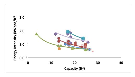
Figure 3 Energy intensity of new ULT freezers from data supplied by manufacturers to the University of California. Each symbol represents a different manufacturer and they show greater disparity than volume relationships, although values have not been independently verified. Differences may result from efficiency or measurement methods.
