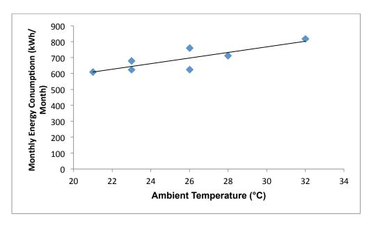
Figure 12 Energy Consumption versus Ambient Temperature for 17.3 ft<sup>3</sup> at set point -80°C for maintained ULT freezers (Gumapas and Simons, 2013)
