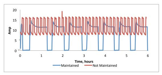
Figure 5 The influence of dust accumulation on ULT freezer filters and condenser fins on amperage for ULT freezers at a set point of -80°C operating in ambient temperatures from 23°C to 25°C (Gumapas and Simons, 2013)
