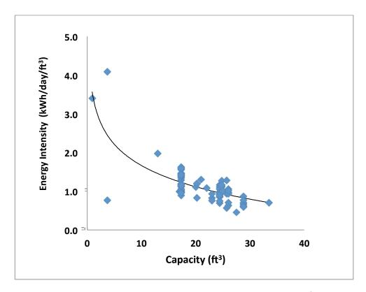
Figure 2 Energy intensity of existing ULT freezers. Freezers smaller than 15 ft<sup>3</sup> use up to three times more energy per volume than 20-25 ft<sup>3</sup> ULT freezers. (Gumapas and Simons, 2013)
