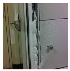
Frosting occurs on any surface with a temperature that is below the dew point of freezing air and below the freezing point of water. Frosting is generally observed on the evaporator coils and the outer gasket seals of the ULT freezer (Figure 7). Frost accumulation inside the freezer or around the freezer door creates gaps in seals, which allow cold air to leak out and warm air to enter the freezer. Frost can also damage the seals on the freezer.
