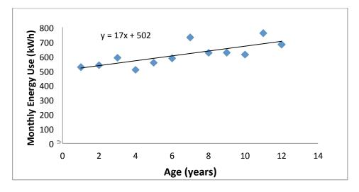
Figure 1 Energy consumption versus age for maintained 17.3 cubic foot (ft³) ULT freezers at a set point of -80°C (Gumapas and Simons, 2013)
