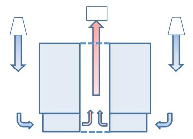
Figure 16 Reject heat management with panels and stratification.
