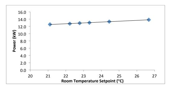
Figure 13 Energy Consumption measured at the electrical panel versus Ambient Temperature for ten ULT freezers (University of California, Davis).
