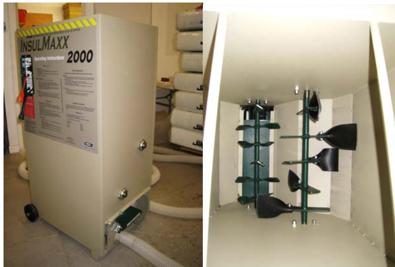
Figure 2. InsulMaxx 2000 all fiber machine (left) with double agitators (right)
