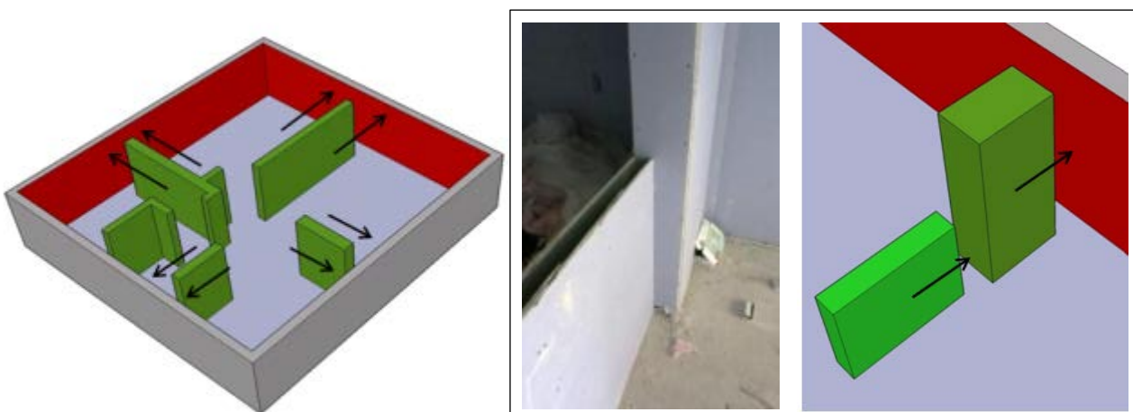
Figure 9. Layered drywall approach. Red surfaces indicate continuous drywall that forms the apartment air barrier. Green shapes indicate interior partitions.
