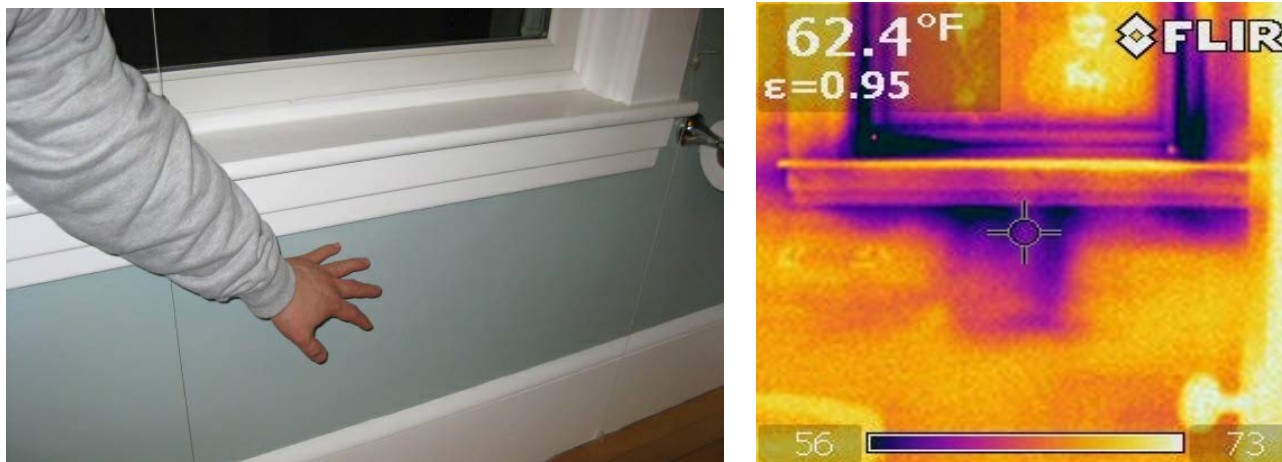
Figure 16. Infrared images of window air leakage at window interior apron trim. Dark colored areas indicate cold surface temperatures from cold outdoor air leaking into the building.
