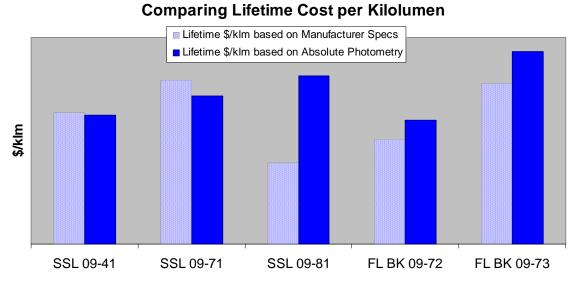
**Figure 6.** Comparative Cost per Kilolumen Based on Manufacturer Performance Data and Based on Results from CALiPER LM-79 Testing (Absolute Photometry)<sup>10</sup>
