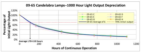
Figure 10c. Rapid Light Output Depreciation for SSL Candelabra Lamp
