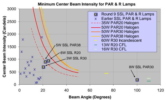
Note: Halogen curves based on draft ENERGY STAR criteria. Incandescent and CFL data points from CALIPER benchmark testing.
