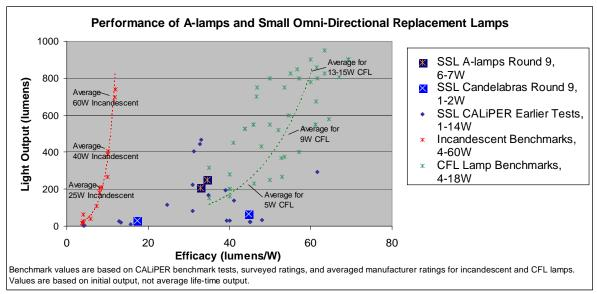
Figure 9. Comparison of A-lamp SSL Products Versus Benchmarked Traditional Lamps
