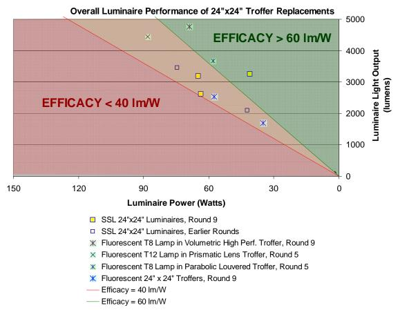
Figure 4. Luminaire Light Output and Power for 2'x2' SSL Fixtures and Fluorescent Troffers
