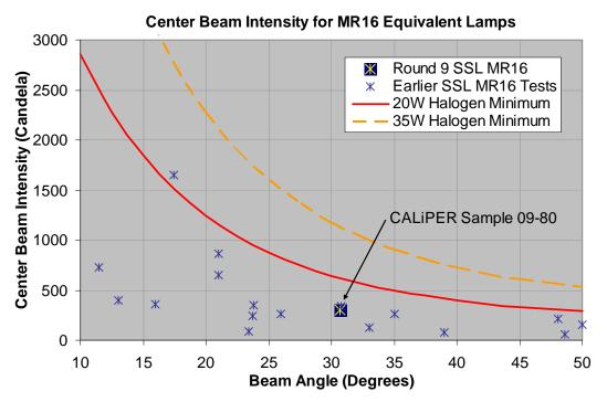
Figure 7. Center Beam Intensity for MR16 SSL Lamps Compared to ENERGY STAR Defined Minimum Center Beam Intensity for Halogen MR16 Lamps (To achieve intensity level of halogen lamps, SSL lamps must fall above the target line for the equivalent wattage they intend to replace.)
