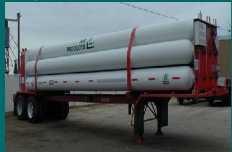
Gaseous hydrogen delivered at ~2600 psig
