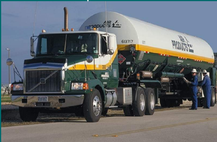
Liquid hydrogen delivered at about -425°F and 100 psig.
