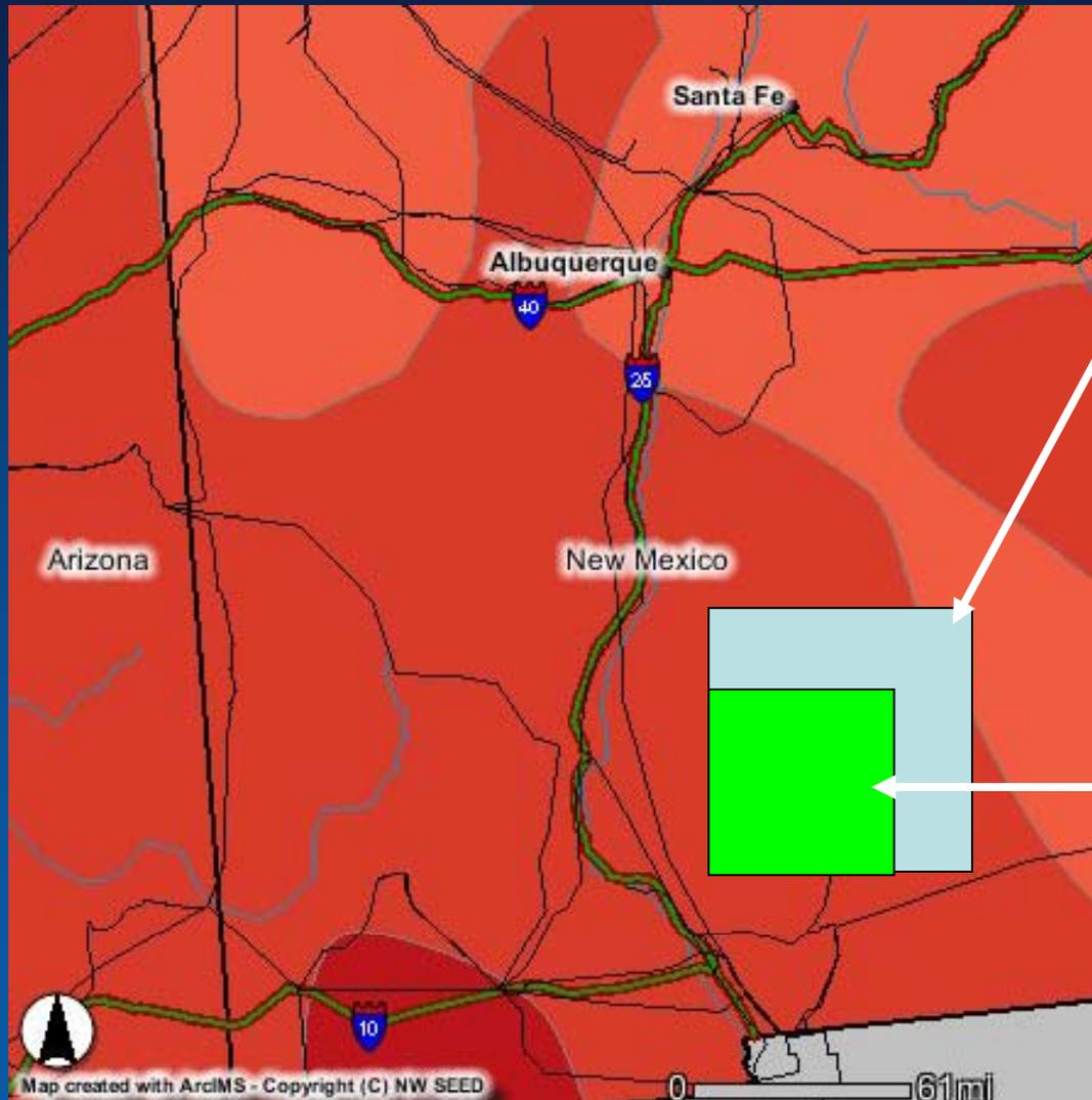
PV panel area to produce hydrogen for current US fleet (10% system, 70% electrolysis efficiency)
