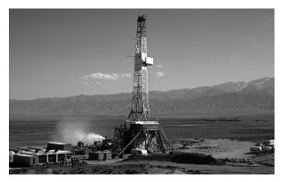
**Getting to the Geothermal Reservoir** If geologists find encouraging signs of deep heat, wells will be drilled. Drill rigs can be small water-well truck-mounted rigs, or large drill rigs like these, erected onsite. Geothermal wells can be drilled over two miles deep. (*Photo courtesy* of Geothermal Education Office, Tiburon, CA)
