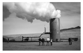
Testing a Geothermal Well
