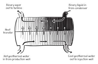
Binary Power Plant Heat Exchanger
