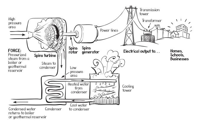
How a Steam-driven Power Plant Works
