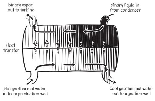
Binary Power Plant Heat Exchanger
