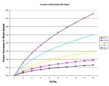
This graph shows two things. As we increase in height (in this case the ratio of  $H/H_{\rm O}$ ) our wind speed increases. It also shows that over rougher surfaces with a higher shear exponent this increase in speed can be dramatic. With a shear value of .4 (suburbs or woods) winds can be 2x faster at 7x the height. The problem is with a high shear factor that these winds may be quite turbulent.
