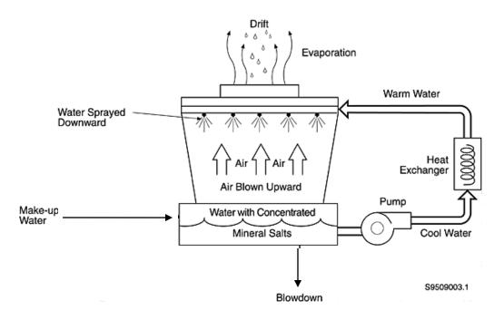
Figure 1: Typical Open-recirculating Cooling System
