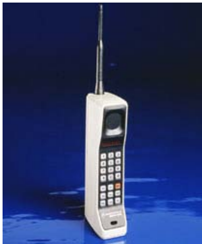
First Cell Phone By Motorola, 1973 12 inches long, 2 lbs, cost $3995
