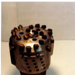
Figure 1.4 - PDC drill bits account for more than one-third of the total footage drilled worldwide.
