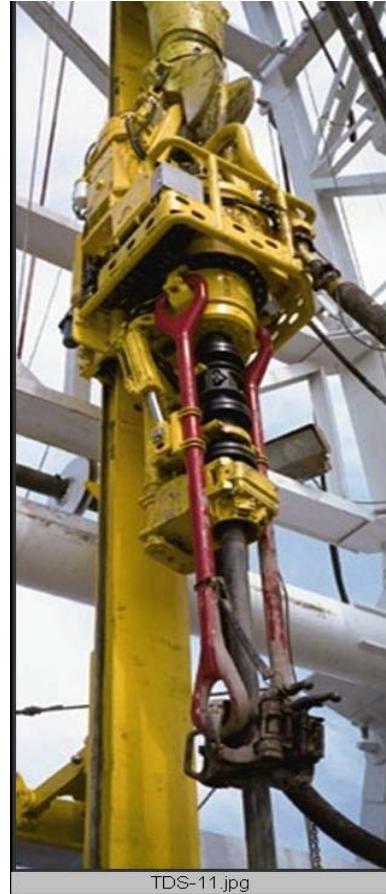
Figure 5 Top drive, photo courtesy of National Oilwell Varco
