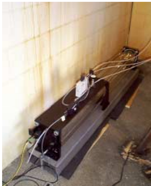
Figure 1. H 2 S Analyzer and Multi-Pass Sampling Cell Deployed Behind Houston Atlas Instrument at NCPA.
