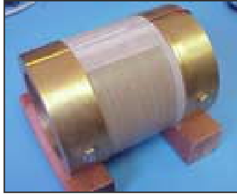
Figure 3. A piezoelectric transmitter for acoustic MWD.
