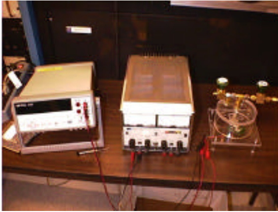
Figure 1. Test Apparatus for Thick Film Hydrogen Sensors.
