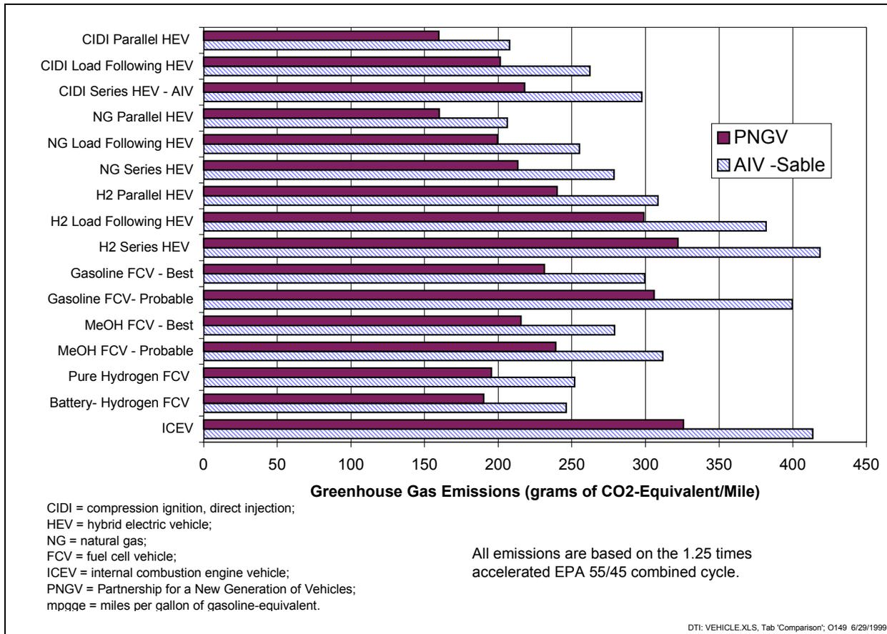
**Figure 3.** Estimated Greenhouse Gas Emissions from Alternative Vehicles
