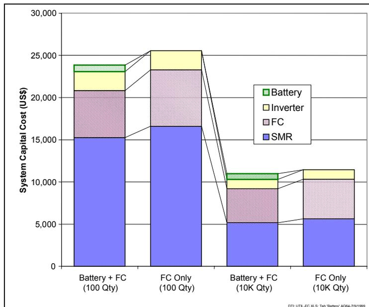
Figure 12. Capital Cost Estimates for a 3.4 kW<sub>e</sub> Fuel Cell System with Battery Peak Power Augmentation
