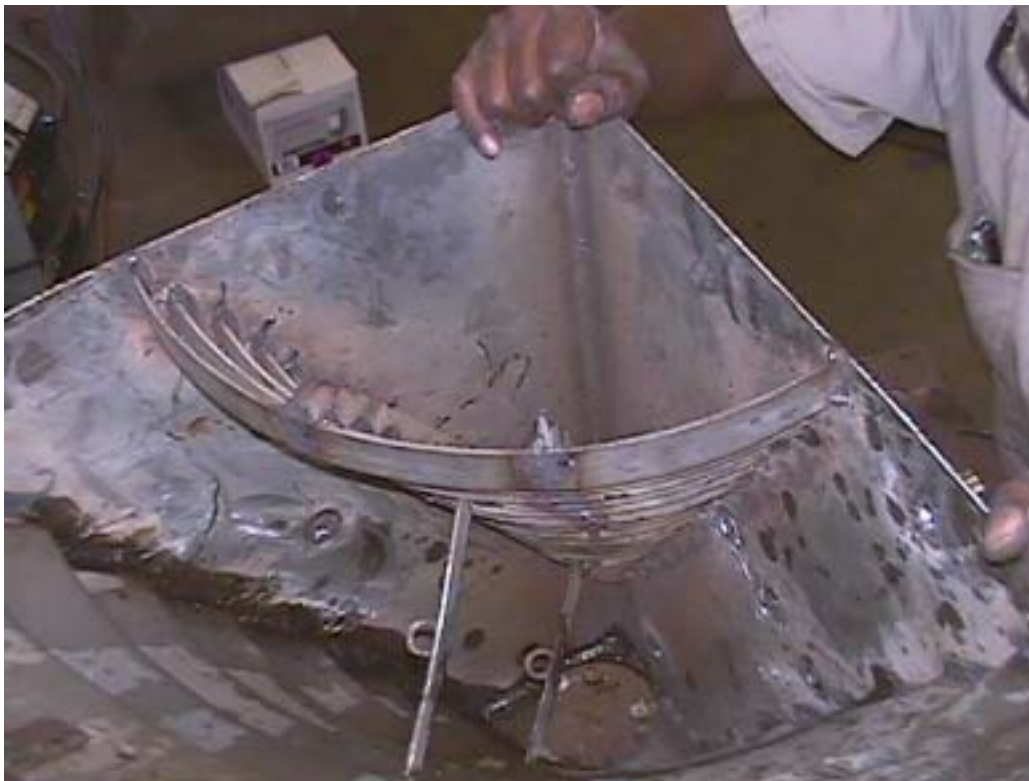
Figure 8: Photograph showing the inside of the cross flow vertical moving bed pyrolysis unit
