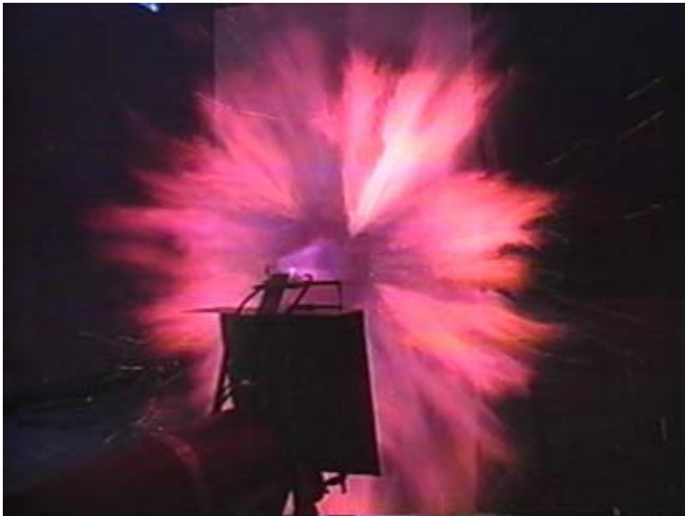
Figure C 2 – Hydrogen flame impingement, early in burn
