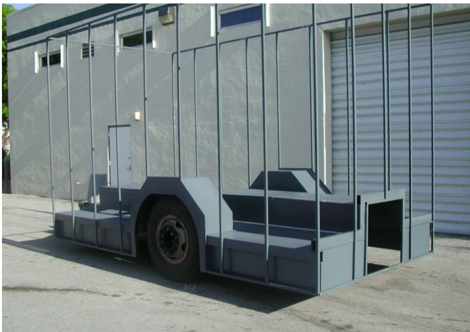
Figure A 20 – Full scale model of front half of bus
