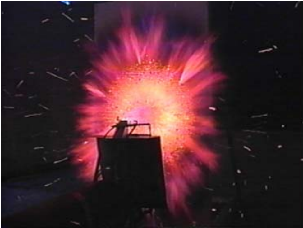
Figure C 3 – Hydrogen flame impingement on gypsum wallboard (paper cover burning)
