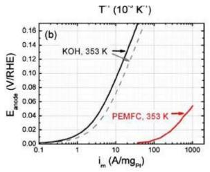
Figure 4. Comparisons of HOR for Pt at high pH and low pH<sup>17</sup>
