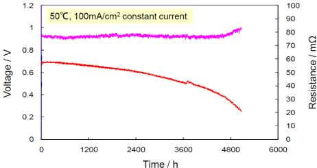
Figure 6. AMFC durability testing at Penn State at 100 mA/cm<sup>2</sup>.
