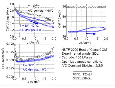
Changes to anode allow high performance operation under challenging conditions – temperature as low as 30 °C
