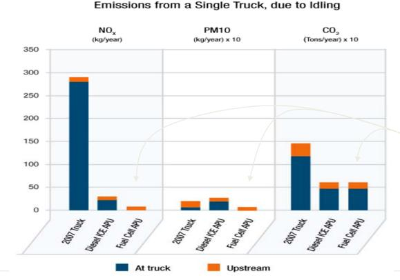
Diesel-powered fuel cell APUs offer significant emissions reductions
