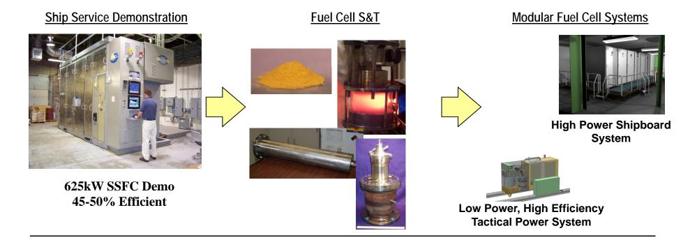
Ship Service Fuel Cell Program Lessons Learned  Enable 3X improvement in volumetric density over SSFC demonstrators
