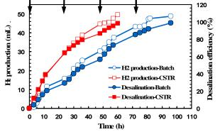
Simultaneous  $H_2$  production (2 m<sup>3</sup>/m<sup>3</sup> d), waste removal (90%), and Desalination (99%) - Energy Positive System
