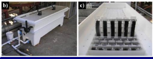
An 1000 L pilot MEC reactor treating winery wastewater and producing H<sub>2</sub>
