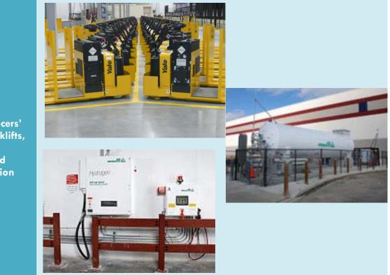
Clockwise: Central Grocers' fuel cell forklifts, hydrogen storage, and fueling station
