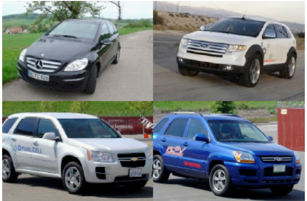
Generation 2 fuel cell vehicles from the National Hydrogen Learning Demonstration. Clockwise, from top left: Daimler F-Cell, Ford Edge, Hyundai-Kia FCEV, GM/Chevrolet Equinox. The demonstration has collected data on 152 vehicles at 24 stations across the country.
