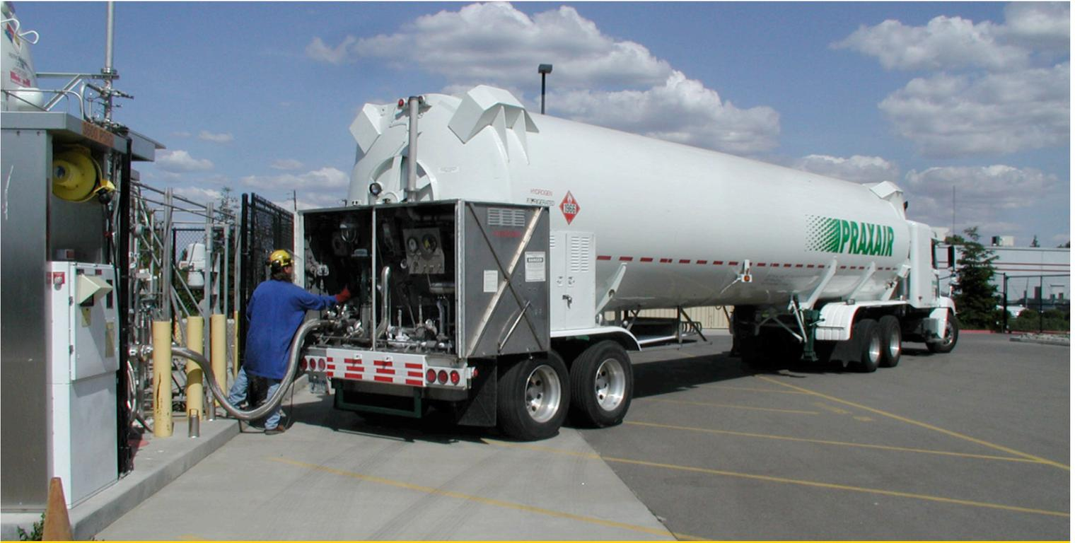
Suppliers currently transport hydrogen by pipeline or over the road using tube trailers and cryogenic liquid hydrogen tankers. For special purposes, liquefied hydrogen is transported by barge. Hydrogen can also be moved using chemical carriers - substances composed of substantial amounts of hydrogen, as well as other elements.
