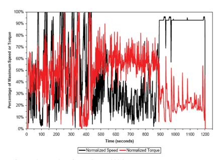
FIGURE 6 Transient Cycle (SWRI 2006)
