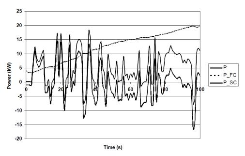
FIGURE 3 Comparison of Input Power of the Fuel Cell System (P\_FC), the Input Power of the Super Capacitor Set (P\_SC), and Power Demand (P) of the Fork Lift Truck
