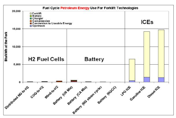
FIGURE 10 Comparison of Petroleum Use by Different Forklift Types
