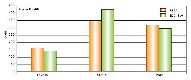
FIGURE 5 Emissions from ULSD and Soy Diesel (in parts per million) (Durbin et al. 2007)
