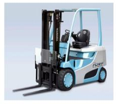
FIGURE 1 Fuel-Cell Forklift (Toyota 2008)
