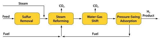
FIGURE 4 Schematic of Steam Methane Reforming to Produce Hydrogen
