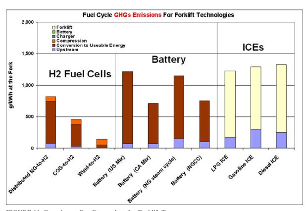
FIGURE 11 Greenhouse Gas Comparison for Forklift Types
