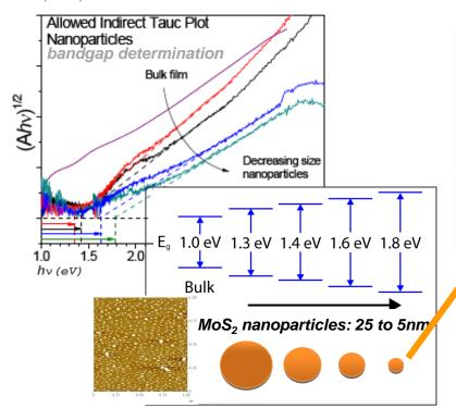
Bandgap blueshift in 5 nm MoS<sub>2</sub> nanoparticles sensitizes catalyst to efficiently absorb light in the solar spectrum
