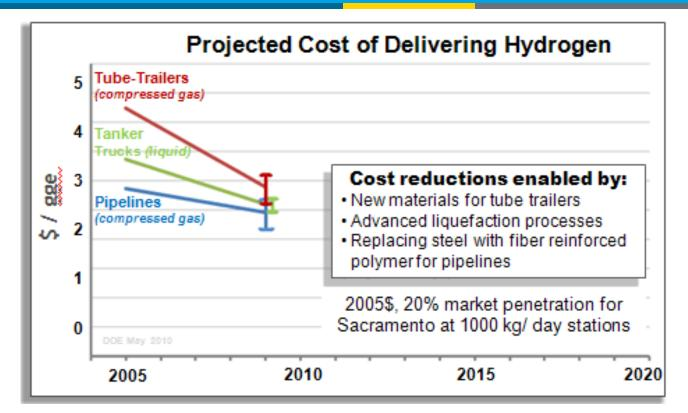
We've reduced the cost of hydrogen delivery\* — ~30% reduction in tube trailer costs >20% reduction in pipeline costs ~15% reduction liquid hydrogen delivery costs
