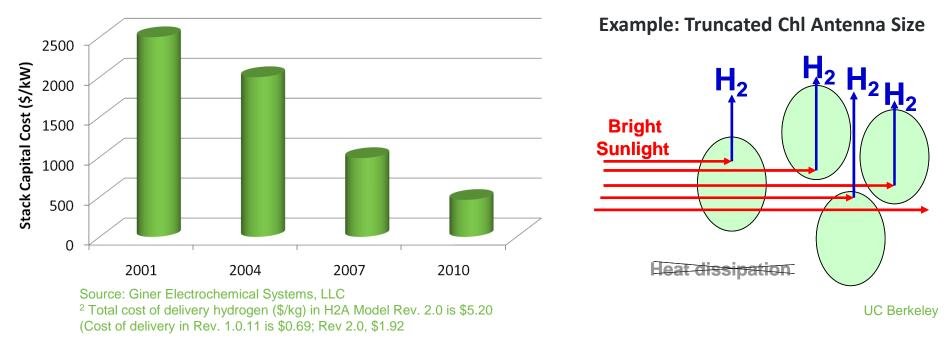
Improved photosynthetic solar –to-chemical energy conversion from 3 to 25% for photobiological hydrogen production by truncating the chlorophyll antenna size (Berkeley)
