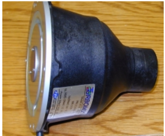
Figure 1. PADT Cathode Air Blower
