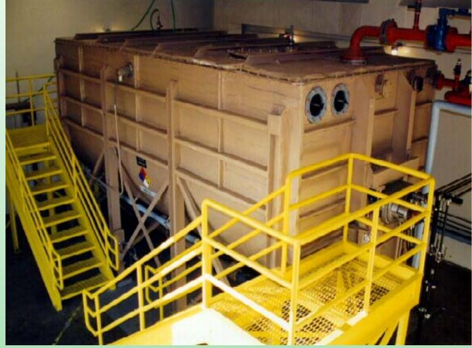
Photo of Plug Flow MSW Digester Courtesy of Pinnacle Biotechnologies Developed at NREL and Sponsored by DOE 1991-2001
