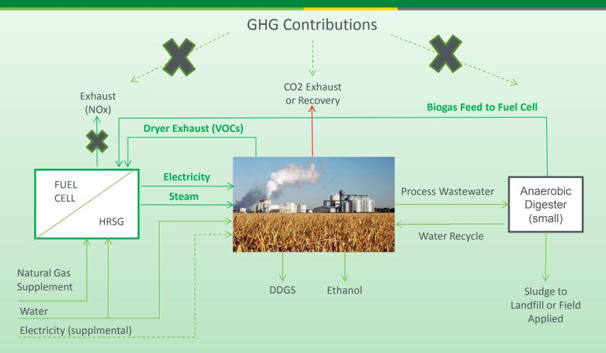
**Dry Mill Ethanol Plant** (Fuel Cell Integration)
