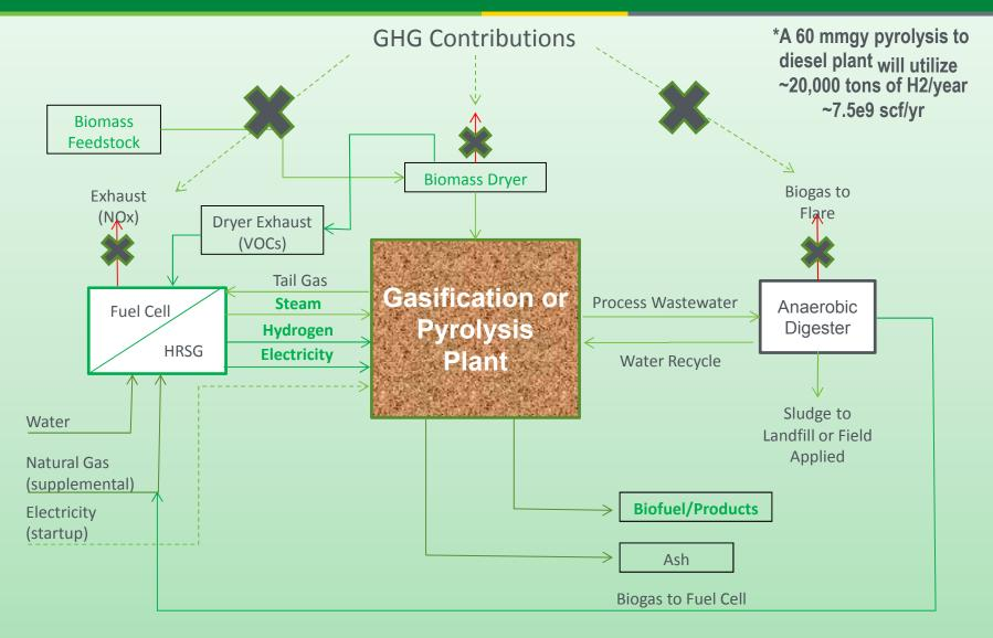
Integrated Biorefinery – Thermochemical (Fuel Cell integration)
