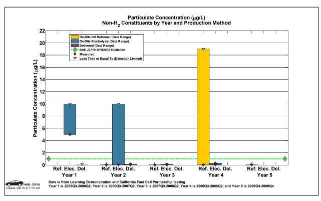
Figure 84: Hydrogen fuel constituents – particulate concentration (CDP28)
