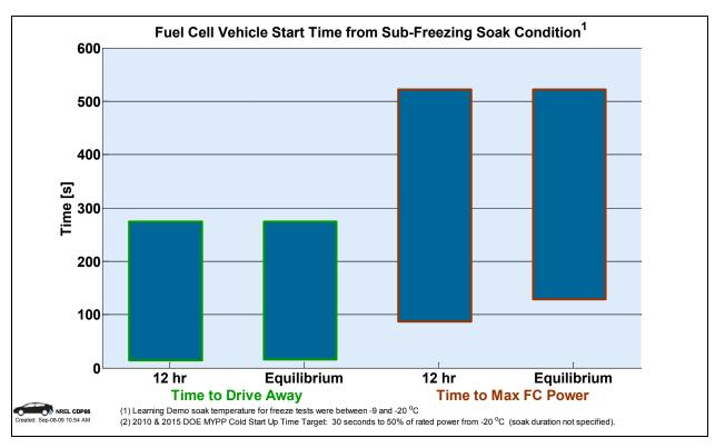
Figure 67: Fuel cell start times from sub-freezing soak conditions (CDP05)
