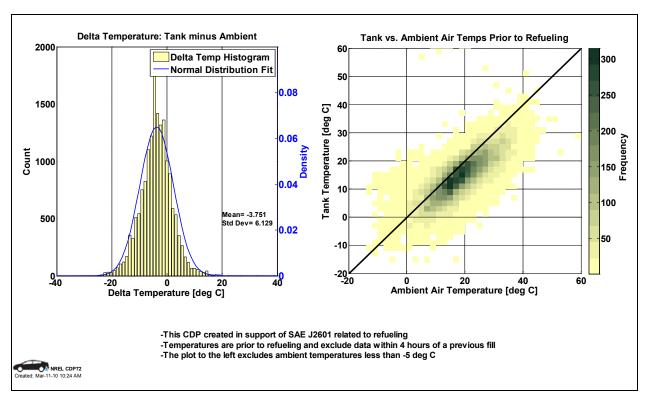
Figure 69: Difference between tank and ambient temperature prior to refueling (CDP72)
