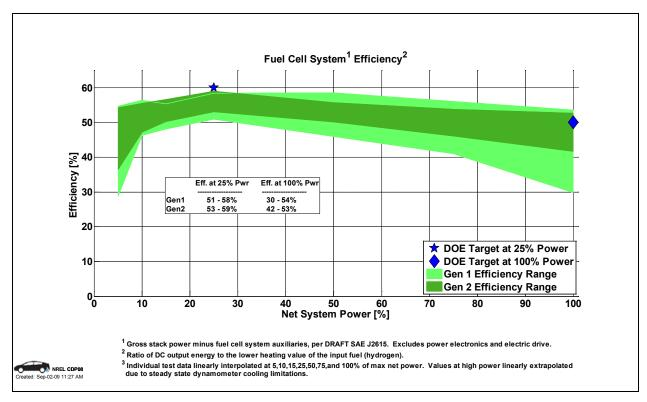
Figure 13: Fuel cell system efficiency (CDP08)
