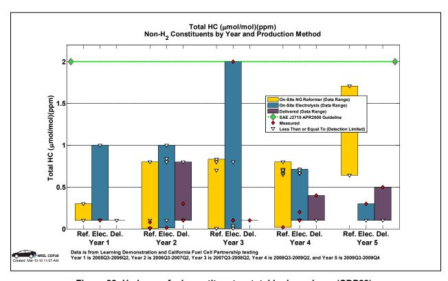
Figure 82: Hydrogen fuel constituents – total hydrocarbons (CDP28)
