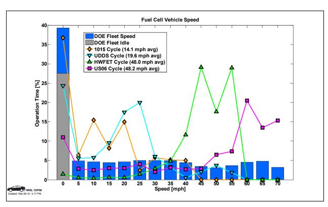
Figure 17: Fuel cell electric vehicle with comparison to standard drive cycles (CDP66)
