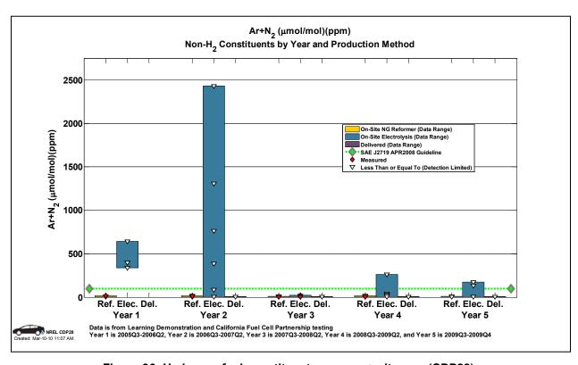
Figure 96: Hydrogen fuel constituents – argon + nitrogen (CDP28)
