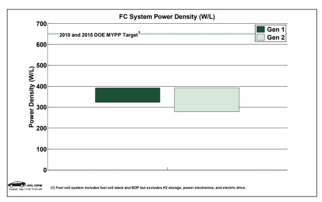
Figure 35: Fuel cell system power density (CDP58)
