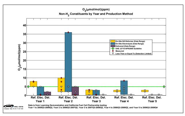
Figure 85: Hydrogen fuel constituents - oxygen (CDP28)
