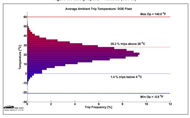
Figure 66: Range of ambient temperature during vehicle operation (CDP21)
