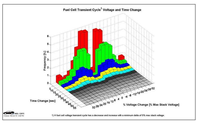
Figure 55: Fuel cell transient voltage and time change (CDP75)
