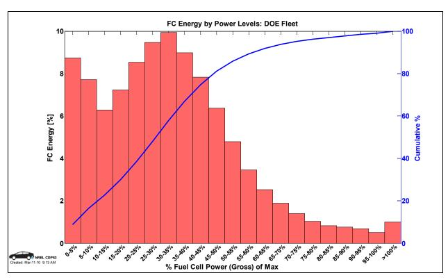
Figure 15: Fuel cell system energy within power levels (CDP53)
