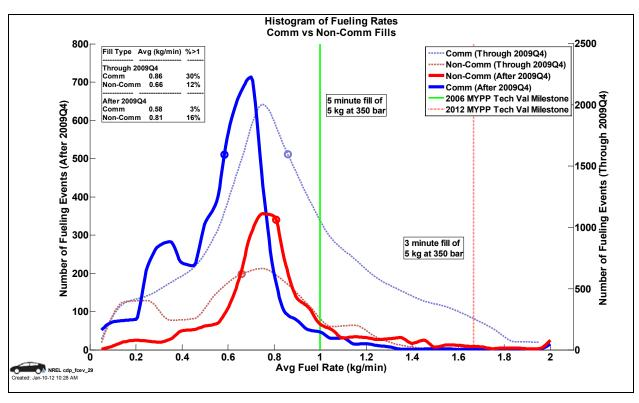
Figure 115: Fueling rates - communication and non-communication fills (CDP29)
