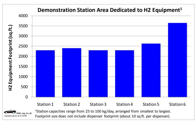
Figure 125: Demonstration hydrogen station equipment footprint (CDP93)
