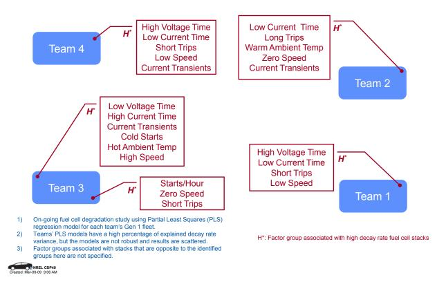
Figure 53: Primary factors affecting Learning Demonstration team fuel cell degradation (CDP49)
