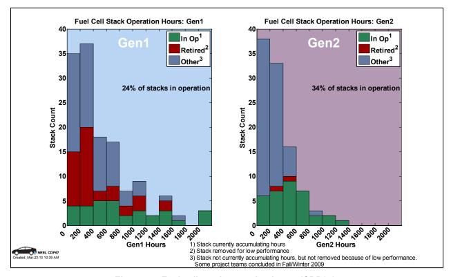
Figure 44: Fuel cell stack operation hours (CDP67)
