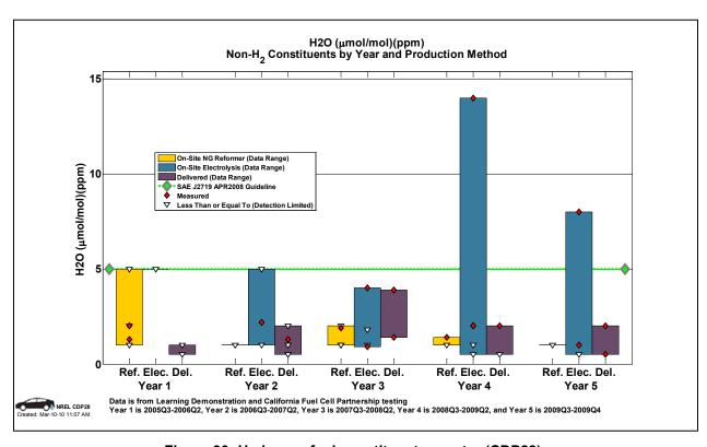
Figure 90: Hydrogen fuel constituents – water (CDP28)
