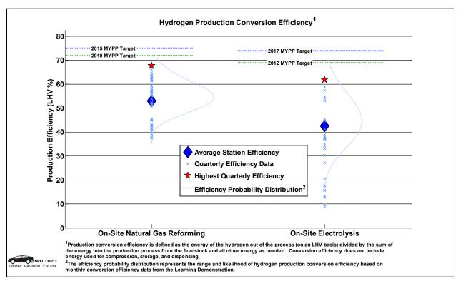
Figure 74: On-site hydrogen production efficiency (CDP13)
