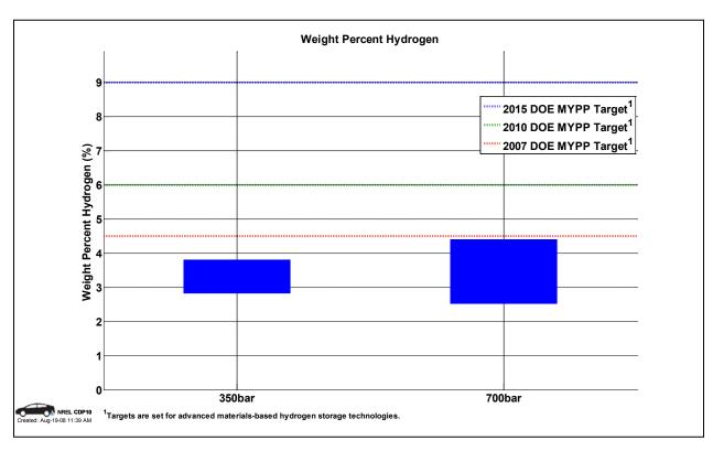
Figure 30: Storage weight % hydrogen (CDP10)
