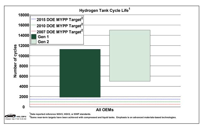
Figure 33: Vehicle hydrogen tank cycle life (CDP12)
