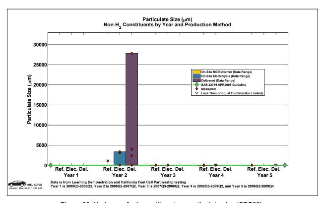
Figure 88: Hydrogen fuel constituents – particulate size (CDP28)
