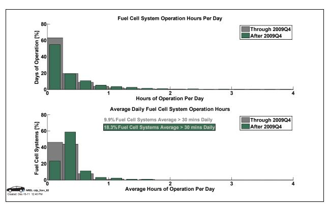
Figure 73: Daily fuel cell operation hours in this automotive application (CDP82)
