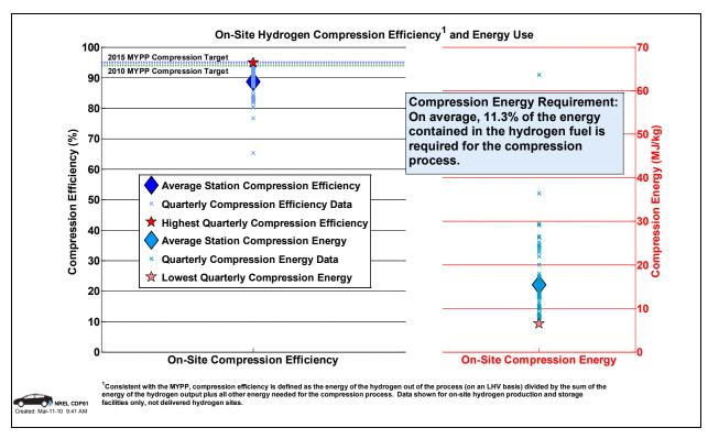
Figure 77: Refueling station compressor efficiency (CDP61)
