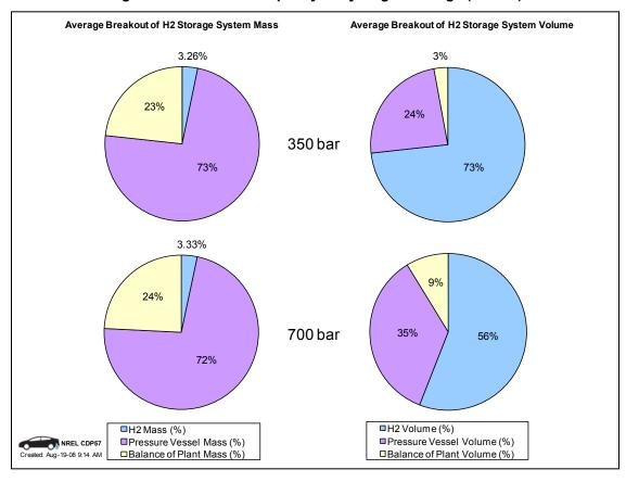
Figure 32: Hydrogen storage system mass and volume breakdown (CDP57)
