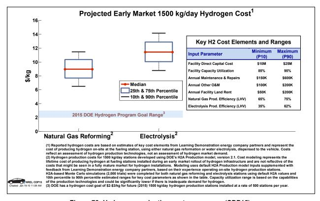
Figure 78: Hydrogen production cost vs. process (CDP15)
