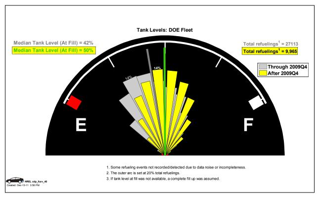
Figure 117: Hydrogen tank level at fueling (CDP40)
