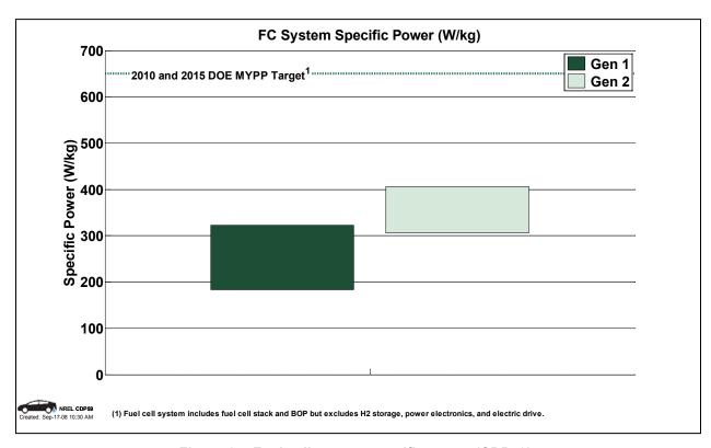
Figure 34: Fuel cell system specific power (CDP59)
