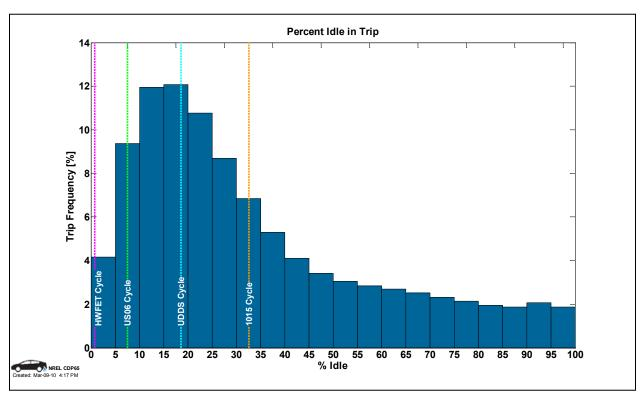
Figure 18: Percent idle in trip with comparison to standard drive cycles (CDP65)
