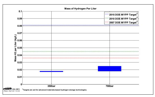
Figure 31: Volumetric capacity of hydrogen storage (CDP11)
