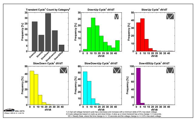
Figure 57: Fuel cell transient rate by cycle category (CDP76)
