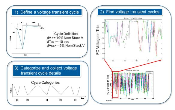
Figure 12: Approach for characterizing voltage transient cycles
