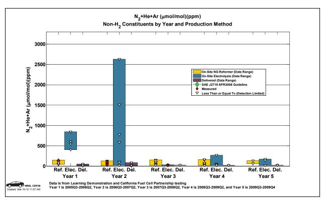
Figure 87: Hydrogen fuel constituents - nitrogen + helium + argon (CDP28)
