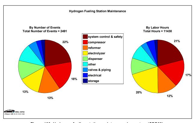
Figure 100: Hydrogen fueling station maintenance by system (CDP63)
