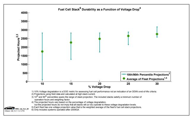
Figure 49: Fuel cell stack durability as a function of voltage drop after 2009Q4 (CDP89)
