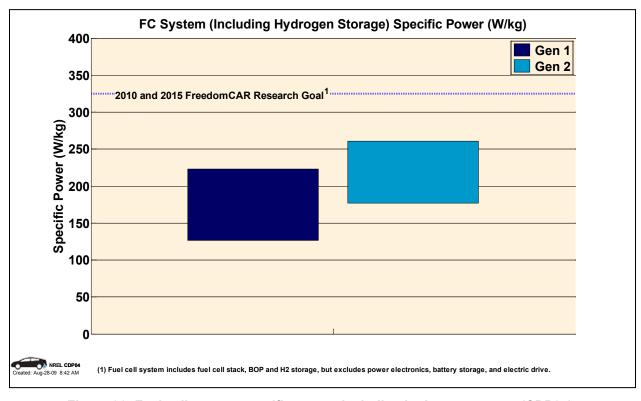
Figure 36: Fuel cell system specific power, including hydrogen storage (CDP04)
