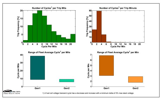
Figure 56: Fuel cell transient cycles by mile and by minute (CDP74)
