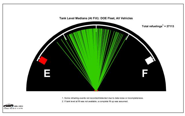
Figure 118: Fueling tank levels – medians (CDP41)
