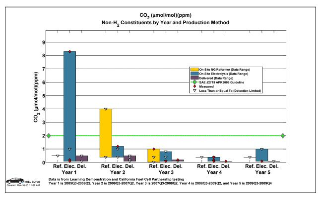
Figure 94: Hydrogen fuel constituents - CO<sub>2</sub> (CDP28)
