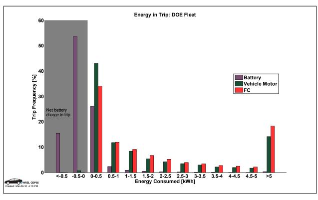
Figure 20: Fuel cell system energy in trips (CDP55)
