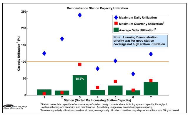
Figure 123: Demonstration station capacity utilization (CDP91)
