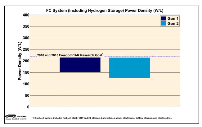
Figure 37: Fuel cell system power density, including hydrogen storage (CDP03)
