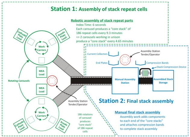
Figure 105. Semi-automated stack assembly work flow diagram
