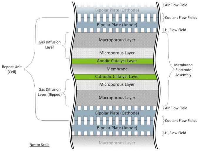
Figure 26. Stack cross-section
