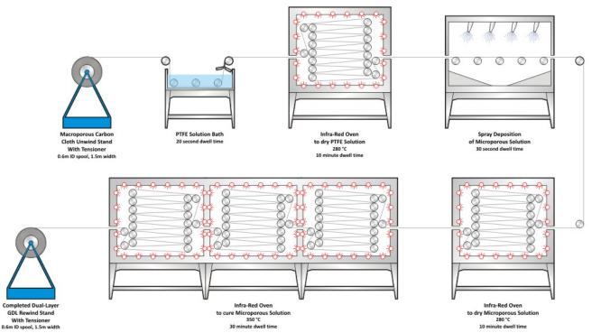
Figure 58. Dual-layer GDL process diagram
