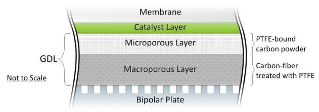
Figure 57. Cross-section of gas diffusion layer in stack
