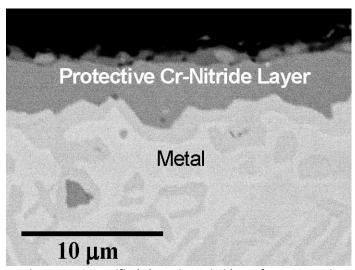
Figure 37. Magnified chromium nitride surface conversion
