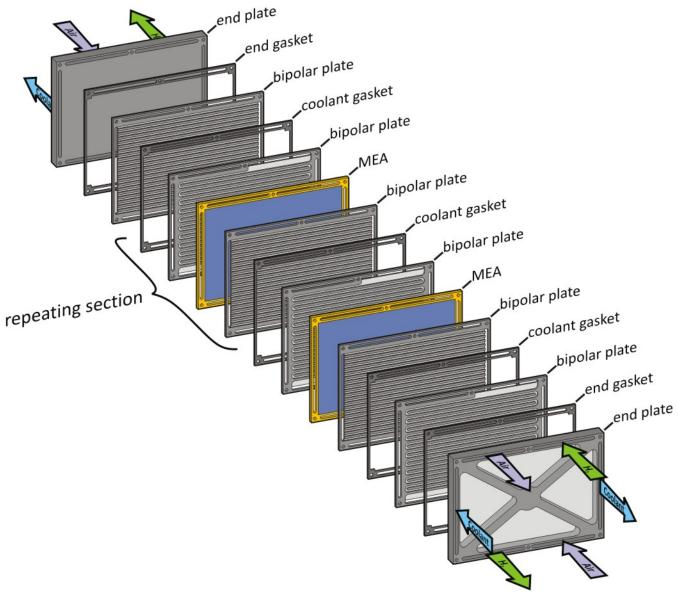
Figure 25. Exploded stack view (abridged to 2 cells for clarity)
