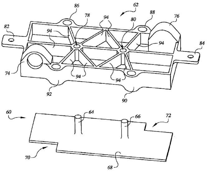
Figure 77. End plate concept, US patent 6,764,786
