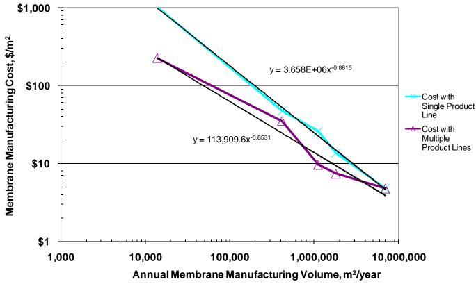
Figure 45. Membrane manufacturing cost vs. annual membrane manufacturing volume
