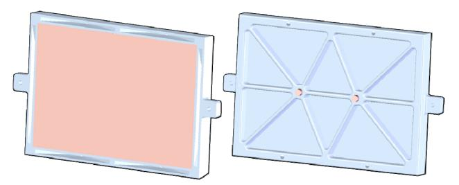
Figure 78. End plate & current collector
