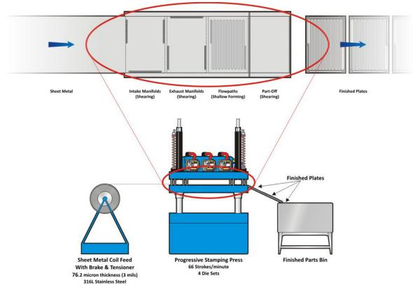
Figure 31. Bipolar plate stamping process diagram
