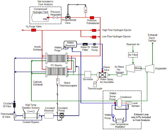
Figure 2. Flow schematic of the 2008 80 kW<sub>net</sub> direct H<sub>2</sub> fuel cell system
