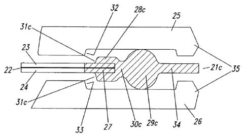
Figure 72. Insertion-molded frame/gasket concept, US patent 7,070,876
