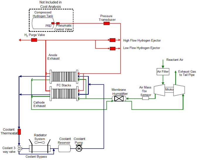
Figure 3. Flow schematic of the 2010 80 kW<sub>net</sub> direct H<sub>2</sub> fuel cell system
