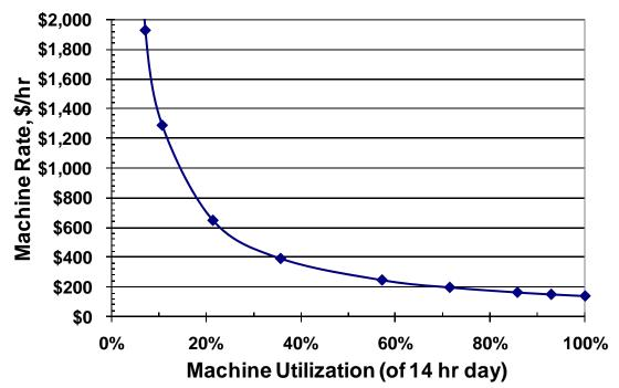
Figure 23. Machine rate vs. machine utilization
