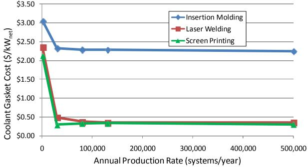
Figure 85. Coolant gasket manufacturing method cost comparison (for 2008 technology)
