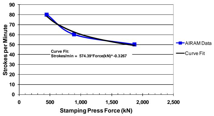
Figure 33. Press speed vs. press force
