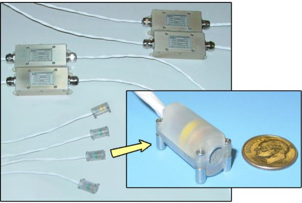
Figure 120. Hydrogen sensors & associated control electronics
