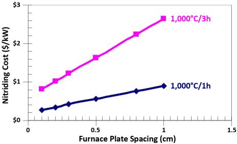
Figure 38. Impact of plate spacing on nitriding cost
