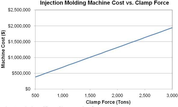
Figure 27. Injection-molding machine cost vs. clamp force
