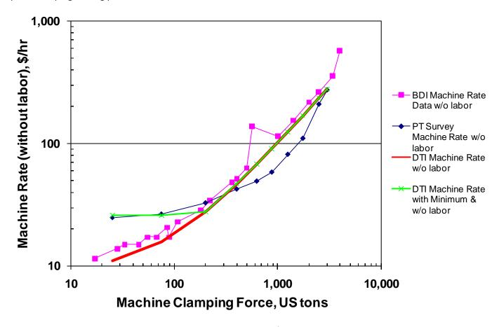
Figure 22. Injection-molding machine rate vs. machine clamping force
