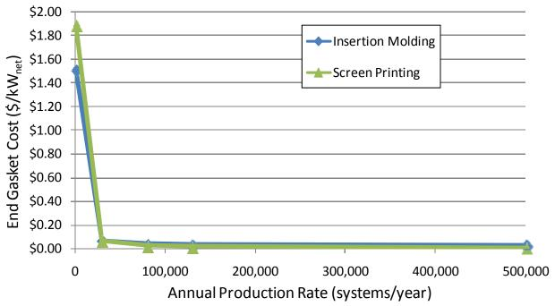
Figure 97. End gasket manufacturing method cost comparison (for 2008 technology)
