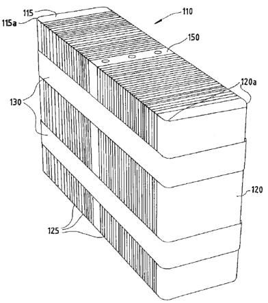
Figure 104. Stack compression bands concept, US patent 5,993,987
