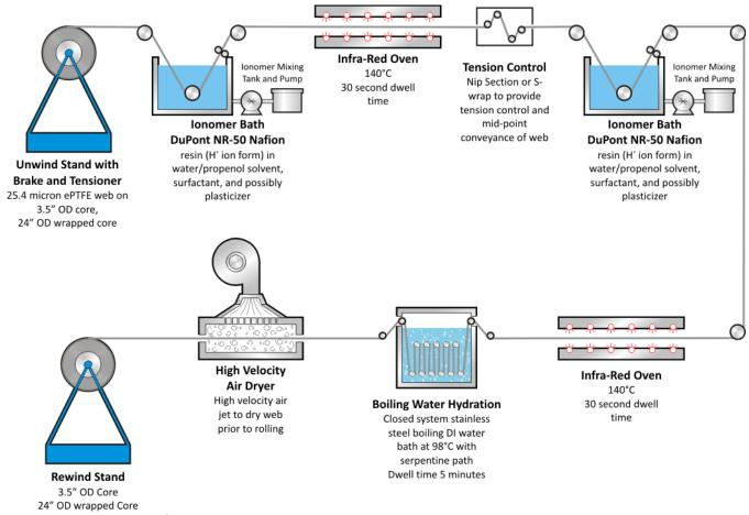
Figure 43. Membrane fabrication process diagram
