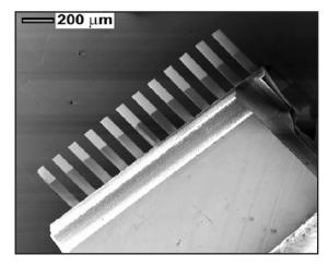
ORNL's Cantilever Array Prior to Alloy Coating
