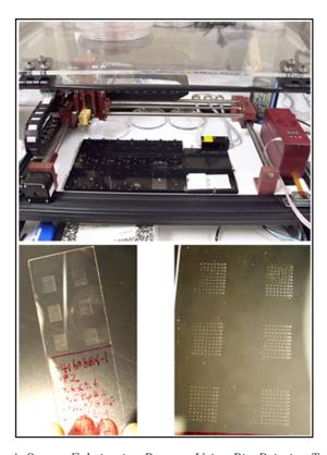
InnoSense's Sensor Fabrication Process Using Pin-Printing Techniques
