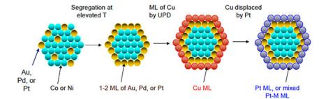
Synthesis Route for BNL's New Class of Cathode Electrocatalysts
