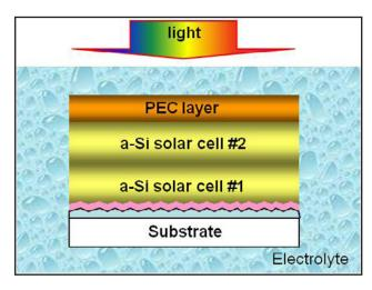
MVS' Monolithic Hybrid PEC Device Powered By a Tandem Solar Cell
