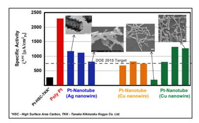
NREL's Pt Electrode Nanostructured Technology
