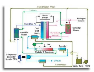
Schematic Diagram of a Hydrogen-Fueled Polymer Electrolyte Fuel Cell System for Automotive Applications
