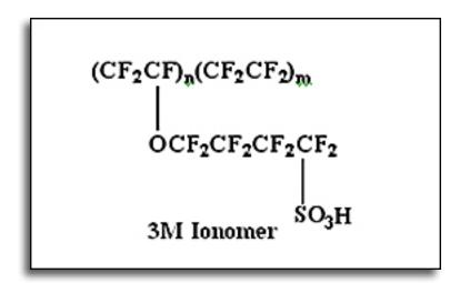
The 3M Ionomer With Lower Equivalent Weight Side Chain than Standard PFSA Ionmers
