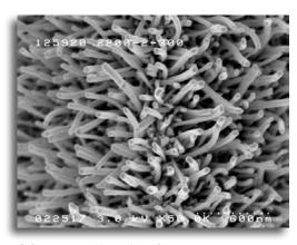
Scanning Electron Micrographs of the New NSTF Catalysts
