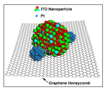
PNNL's Cathode Support Showing Triple Junction Formation
