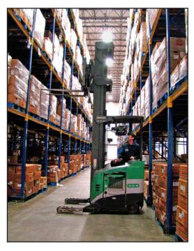
Class 2 Forklift Powered by Nuvera's PowerEdge Fuel Cell System
