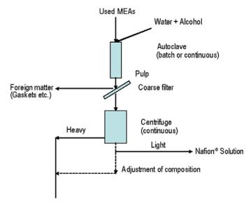
Ion Power's Recycling Process for MEAs
