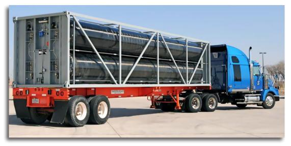
Lincoln Composites' 3,600 psi TITAN<sup>TM</sup> Tank and Frame System
