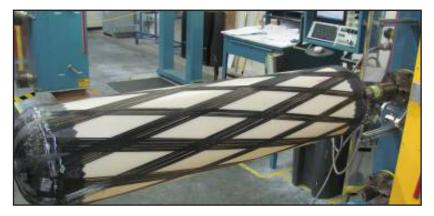
Quantum's Hybrid Manufacturing Technology for Pressure Vessels
