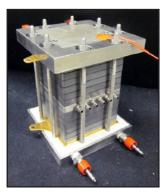
RPI's Test Fuel Cell Stack Using 50 cm<sup>2</sup> MEAs
