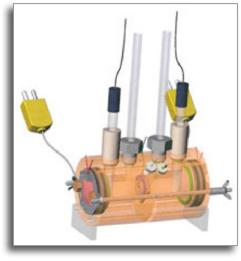
The Corrosion Test Cell Unit
