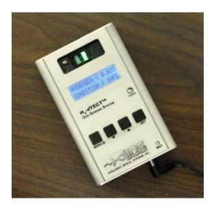
*IOS's Prototype H*<sub>2</sub>-dTECT Hydrogen Sensor
