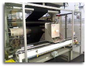
BASF's High-Speed Coating Machine with XRF Monitoring
