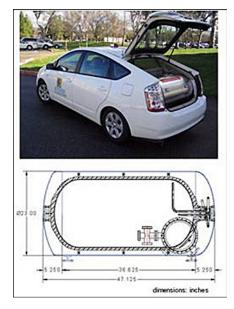
LLNL's Cryo-Compressed Hydrogen Storage Vessel
