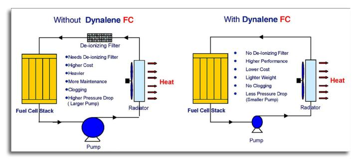
Comparison of Basic De-Ionized Water/Glycol System with Dynalene FC System
