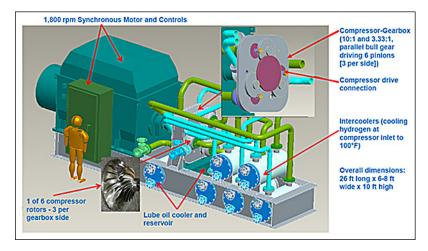
Concepts NREC's Centrifugal Hydrogen Pipeline Gas Compressor
