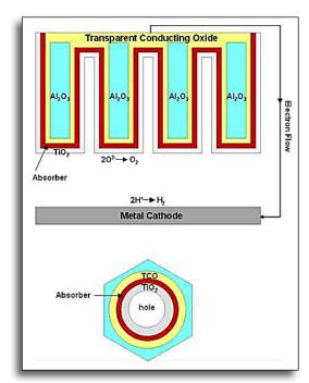
Schematic of Synkera's Nanotube Array with Integrated Absorber
