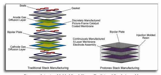
Protonex Injection-Molded Stack Versus Traditional Stack Assembly
