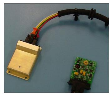
Makel's Low-Cost Hydrogen Sensor for Transportation Safety
