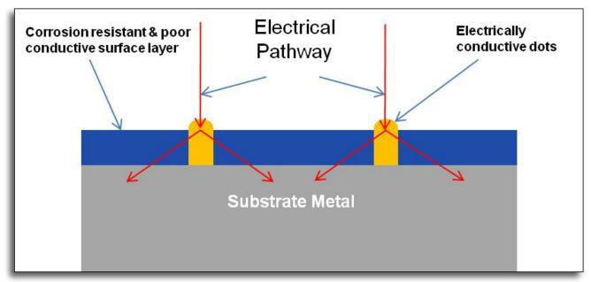
TreadStone's Corrosion-Resistant Metal Plate Design
