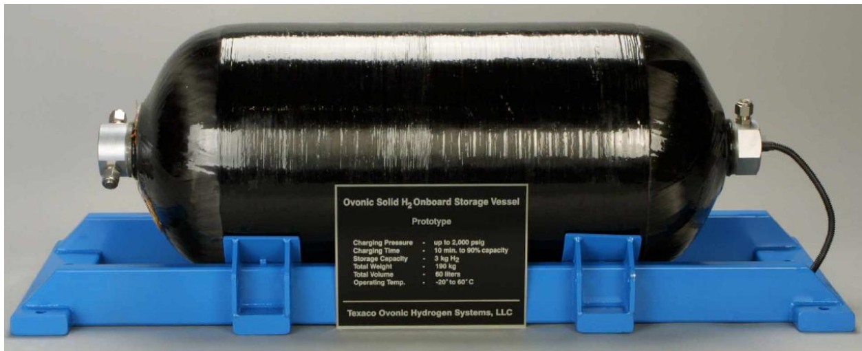
Figure 12: Picture of Ovonic metal hydride storage tank. The nameplate indicates the system shown can store 3 kg (6.6 lb) of hydrogen, has a mass of 190 kg (419 lb), and a volume of 60 L (2.1 ft 3 ). From Chao et al. [36], see for more details.
