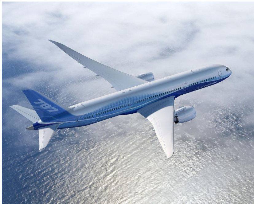
Figure 1: The Boeing 787-8 is a “more electric airplane” with many of the conventional systems converted to electric power. This results in a high on-board electric generating capacity (nearly 1.5 MW). Image ©Boeing, used with permission.
