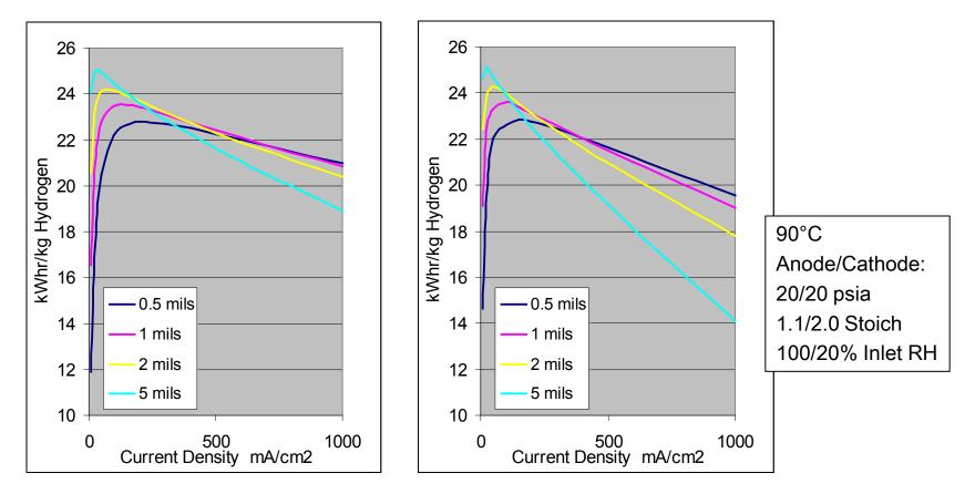
With current PFSA membranes it is not possible to operate high pressure electrolysis with a thin membrane
