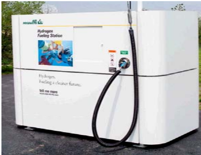
Air Products Series 100E Compression, Storage, Dispensing Module ~9'x4'x6' Nominal Fill Pressure: 350 barg (~5,000 psig) 3 Bank Cascade H 2 Storage
