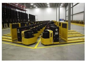
Central Grocers has purchased 221 Yale forklifts powered by PlugPower GenDrive PEM fuel cells for their distribution center in Joliet, Illinois. Air Products is providing the hydrogen gas and fueling stations.
