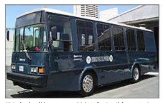
This fuel cell bus uses a 20 kW fuel cell from Hydrogenics. The bus originally was used in a yearlong demonstration at Hickman Air Force Base in Honolulu, Hawai'i. It has since entered into regular service on the base.
