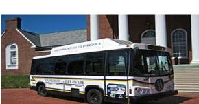
The University of Delaware's Department of Mechanical Engineering conducts research on two fuel cell buses that operate along normal campus routes. The 20 kW fuel cells are from Ballard Power Systems.
