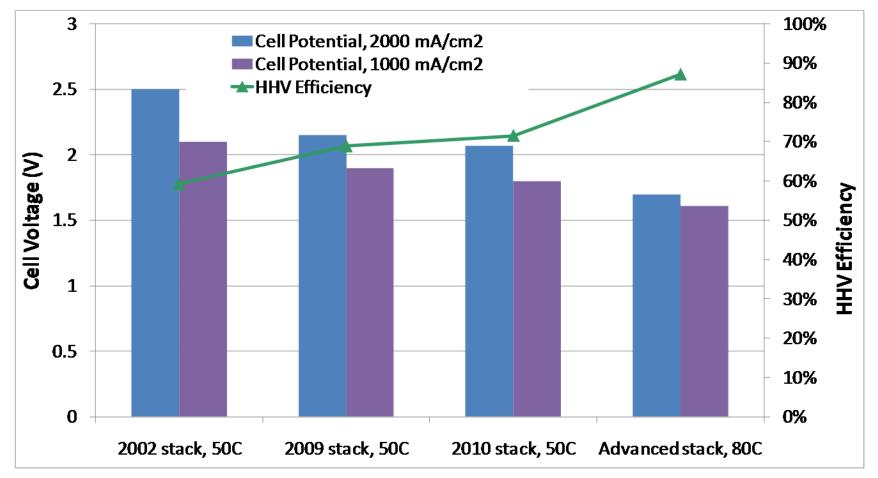
Improvements have enabled double the current density at the same cell voltage over 3 design generations
