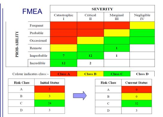
System design improvements and the use of a Dome eliminate the highest severity cases related to hydrogen ignition (Class A), & electrocution (Class B)
