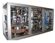
12 Cells - 0.17 ft<sup>2</sup> Cells/Stack 6-kW Electrolyzer 40 SCFH-H<sub>2</sub> (~0.1 kg-H<sub>2</sub>/hr) High Current Density (1300-1500 A/ft<sup>2</sup>) 1000 psi H<sub>2</sub>/Ambient O<sub>2</sub> No High-Pressure Water Feed Pump or **Containment Vessel** Volume 12.5ft<sup>3</sup>
