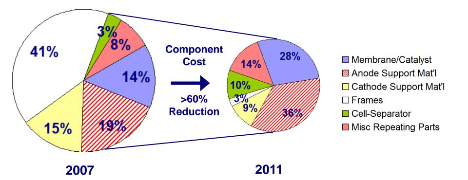
•During DOE funding periods there has been significant cost reductions via new manufacturing techniques •Anode Support Material & MEAs (membrane & catalyst) now dominate cost of the electrolyzer stack 17
