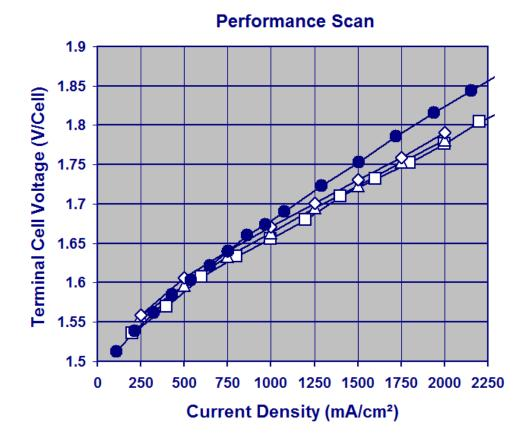
**Test Conditions:** 80°C 320-330 psig Cathode (H<sub>2</sub>) 20 psig Anode (H<sub>2</sub>O/O<sub>2</sub>)
