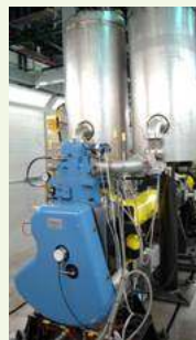
Fig 4. Argonne's nitrogen enrichment tests on a single cylinder research engine.
