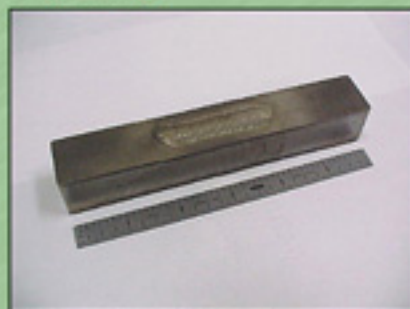
Multi-pass welds made in cast bars confirm that some Ni 3 Si alloys have excellent weldability
