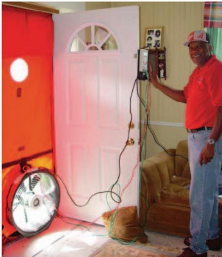
Weatherization technicians use the blower door test to measure the air tightness of building envelopes and diagnose air leakage problems in a home.
