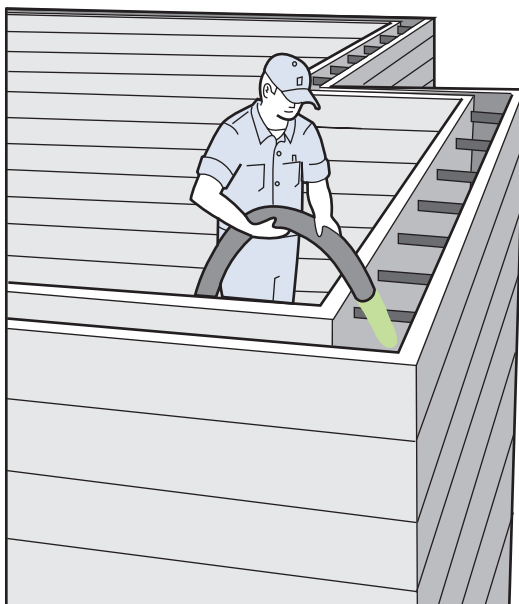
Concrete Being Pumped into the Wall Cavity of an Insulated Foam Home
