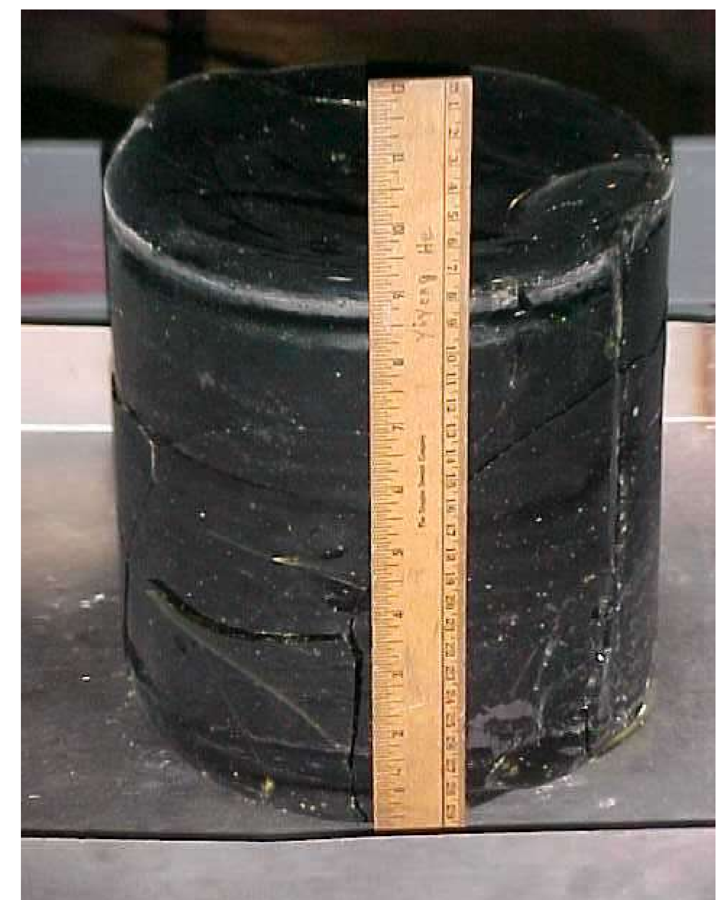
Simulated nuclear-waste glass cylinder (~8000 cm 3 ) melted at 1200 C
