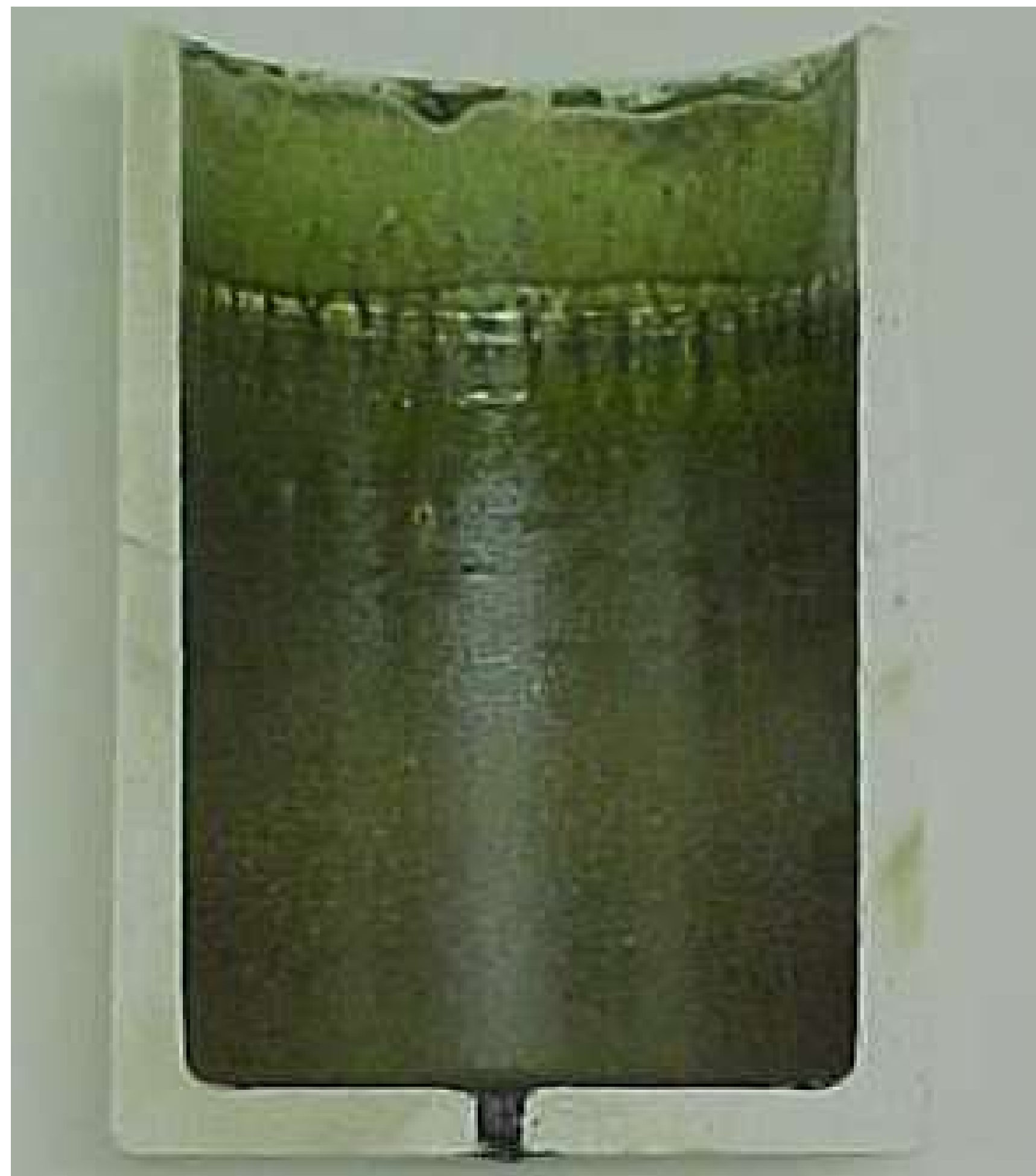
Longitudinal cross-section of a commercially available alumino-silicate crucible after melting ~100 lbs of iron phosphate glass.
