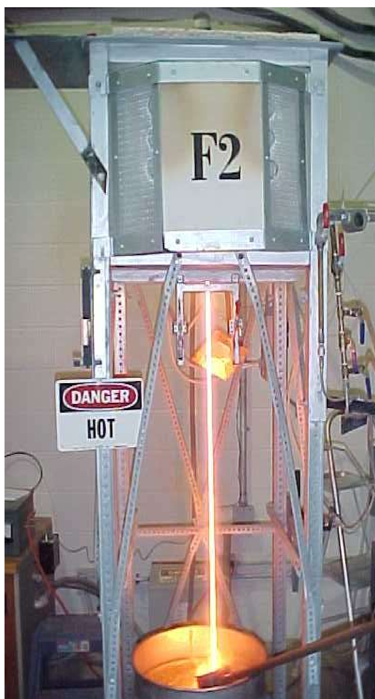
Molten ARP-86 iron phosphate glass being bottom drained
