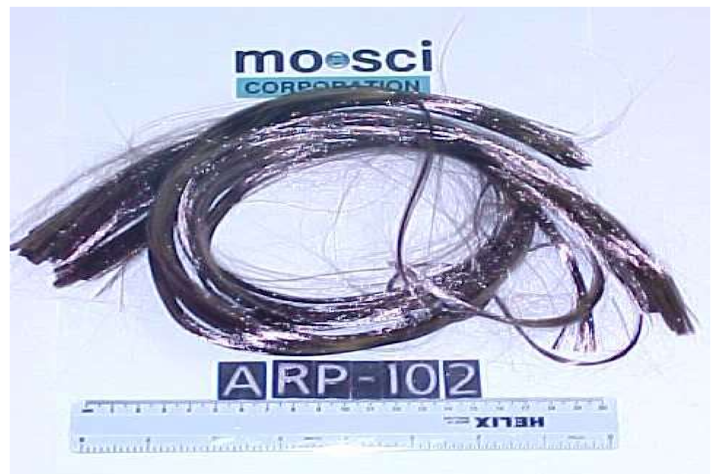
ARP-102 iron phosphate 15-micron glass fiber pulled continuously from one-hole stainless steel bushing at 900 C for 2.5 h
