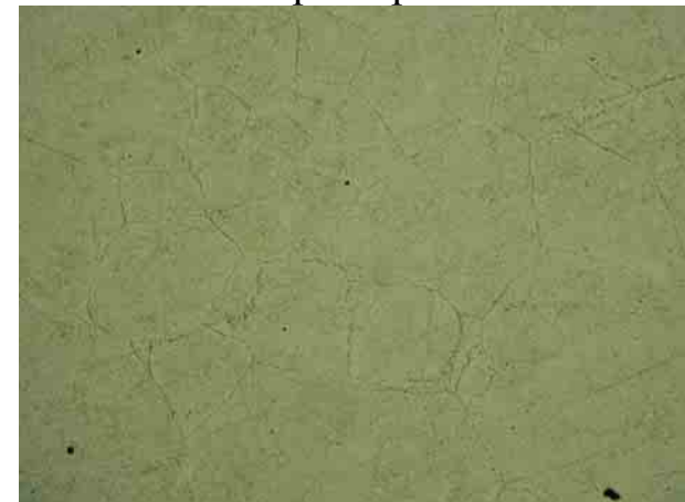
Spray formed. Forced convection cooled. Interior
