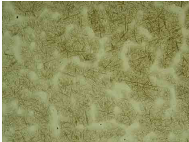
Spray formed. Free convection cooled. Interior
