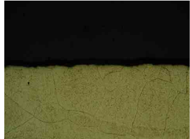
Spray formed. Free convection cooled. Deposit/pattern interface
