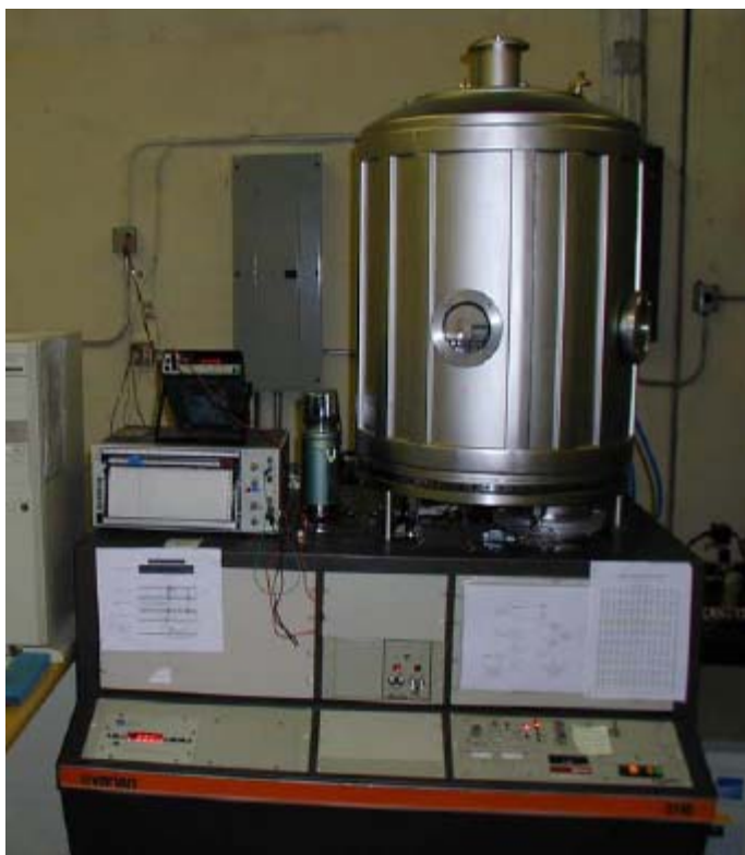
A heat meter developed by Applied Science Laboratories was used for high-temperature thermal conductivity measurement of a large sample (15 by 15 centimeters).
